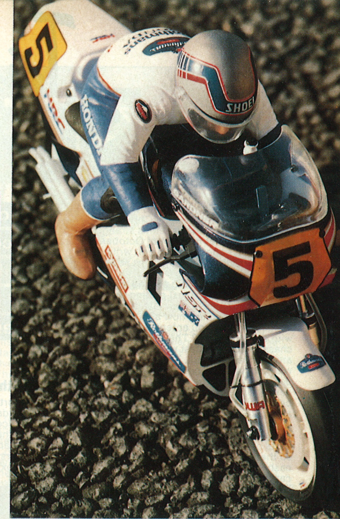
Below: The original kit front forks are replaced with these 'Option House' accessories available from Kyosho. The new units (as described in "On Test") are oil filled and work very well. The front discs are plastic and look great if painted properly.
