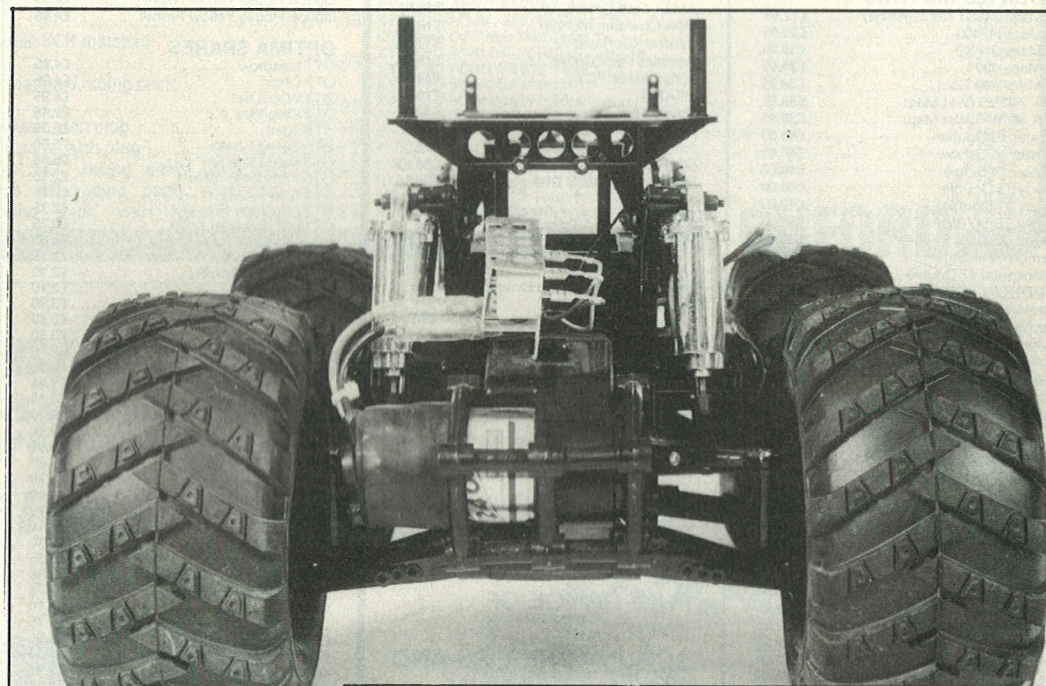
The resistor sits at the rear above the Le Mans motor. Right: centre 'Tub' houses the radio equipment and three speed controller.
