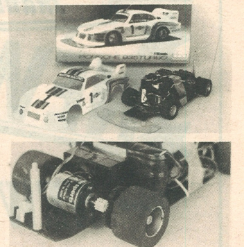
TOP: The Porsche 935 Turbo box, body and chassis with radio. ABOVE: The sidewinder drive of the 1:20 scale model is reminiscent of slotcars.
