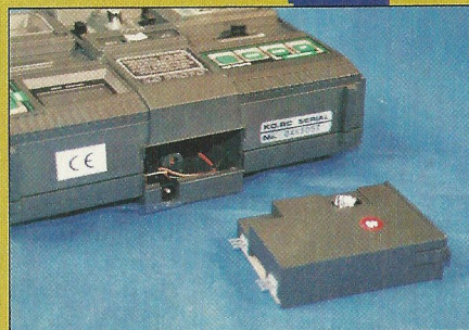
Crystal changes can be a little difficult, the "module" removal not being particularly easy.
