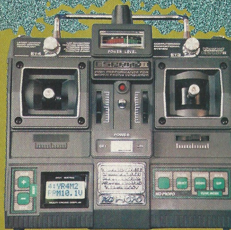
The LCD display is very clear, the adjustable contrast allowing it to be seen even in the brightest conditions.
