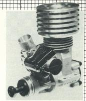
ensure some ventilation to the plug area by provision of drilled hole(s) in the large recessed heat sink heads which have horizontal finning.
