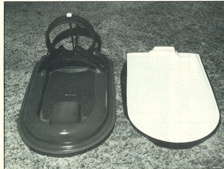
A simple servo pad keeps all in place, note how close the propeller/duct relationship is.
