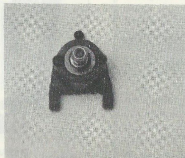
Rear stub axle assembly.
