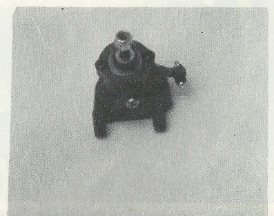
Front drive—stub axle and suspension assembly.
