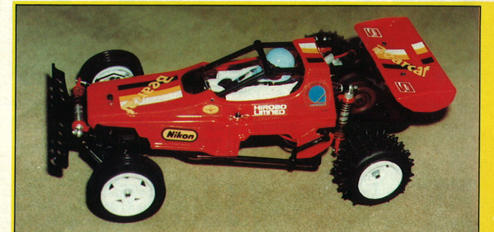
Low slung yet light lexan bodyshell.
