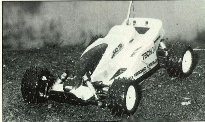
② Coil over oil units are fully adjustable for length and tension.
