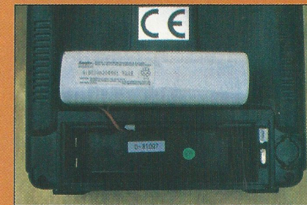
Rear view of the transmitter with the battery cover removed.
