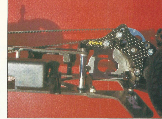
Gearbox stiffening plate.
