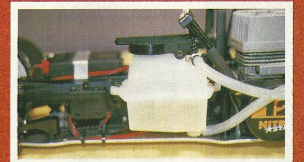
I replaced the kit fuel pipe with some thicker Associated line.
