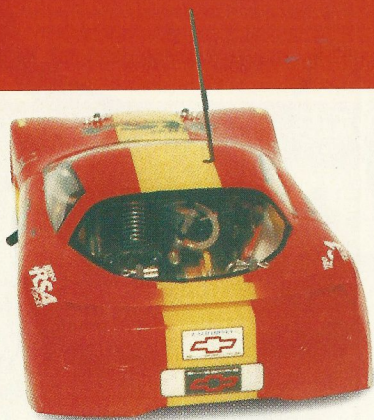
The rear window will need to be part cut out for engine cooling.
