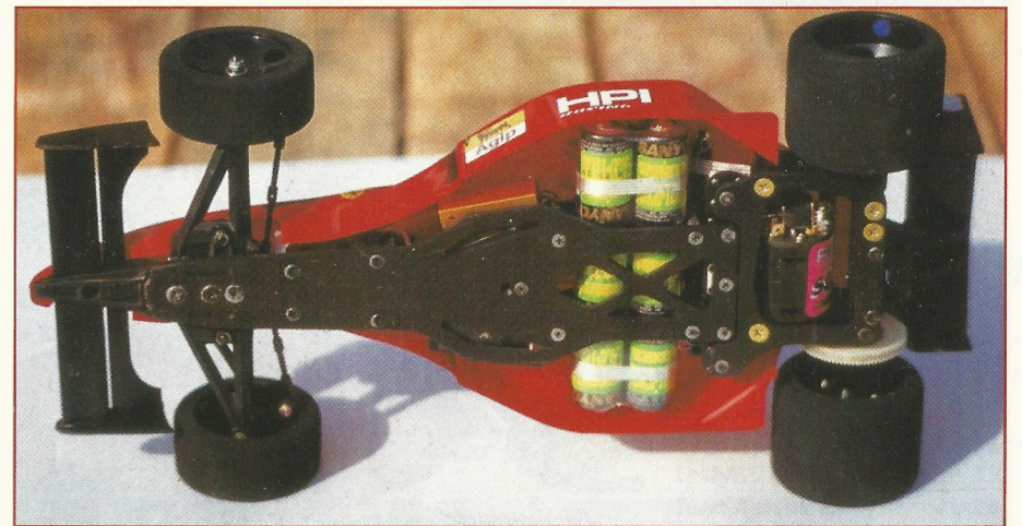
What the track se's. Note the cells are retained by glass-fibre reinforced tape.
