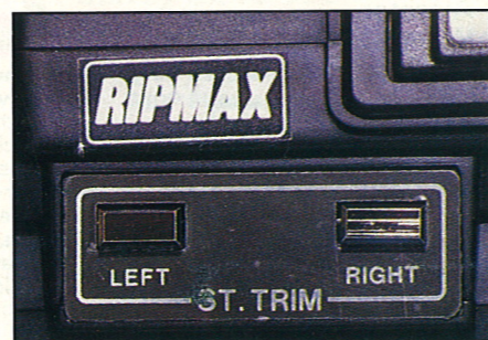
Neutral adjuster gives different amount of throw on the trigger.
