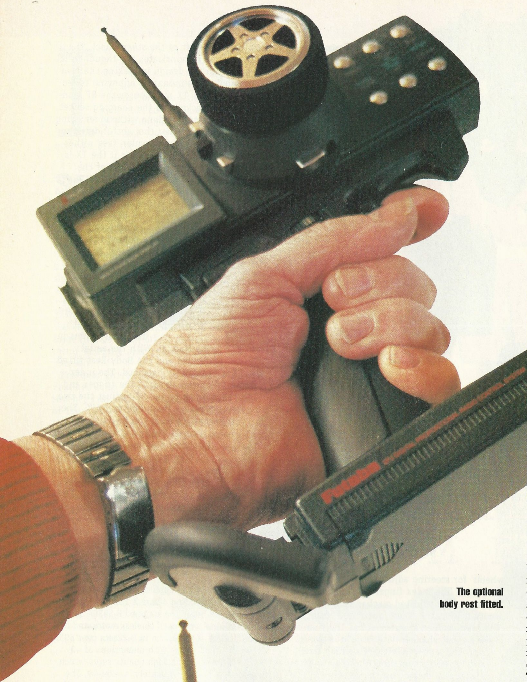
This pic shows the two steering dials above the grip, the throttle digital trim to the left of the steering wheel and the wheel tension access to the right of the PSB.
