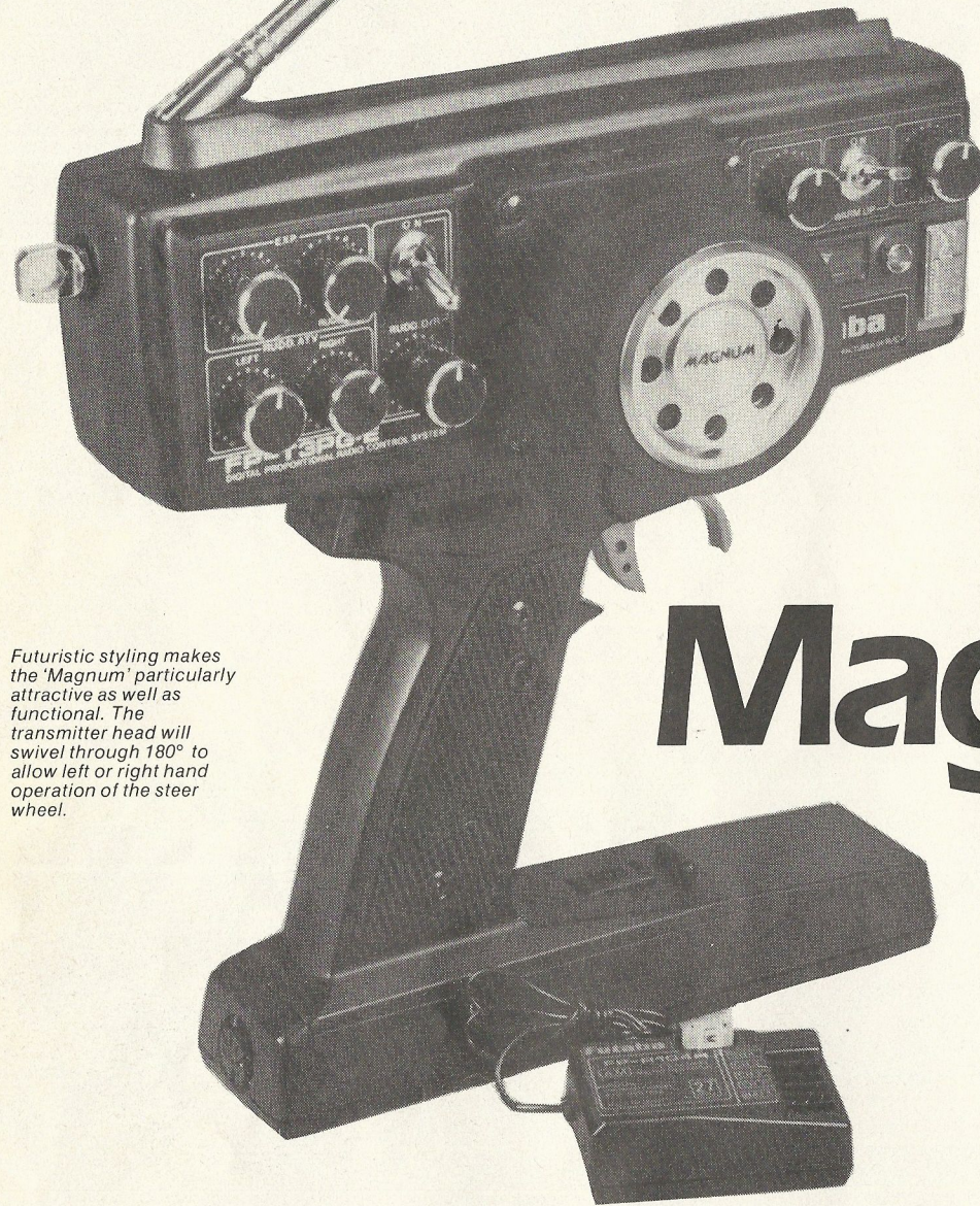
Below: the 'Magnum' transmitter head affords the user very quick control adjustment of all the vital functions. The aerial folds away flush with the transmitter top out of harm's way. The steer wheel itself can also be adjusted for spring tension so that the driver can 'feel' the steering.
