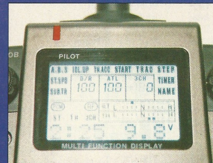
Close up on the Steering & Throttle trim settings above the TX voltage display
