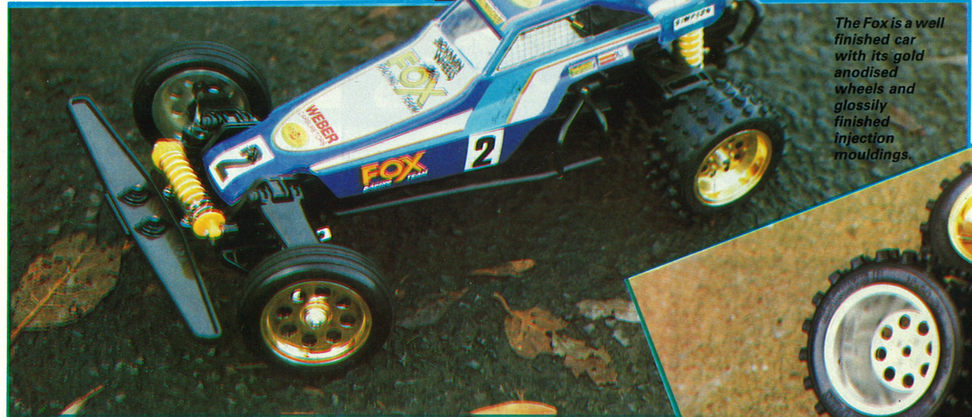
The Fox features a unique variable rate damping system, using three different flow restriction pistons.
