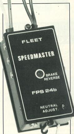
Technically the F.P.S. - 24b is a high performance unit which uses six F.E.T.s forward and three Darlingtons for reverse. Maximum forward current is 144 amps continuous short term, 32 amps continuous short term. Voltage drop across the unit is a mere 0.07 volts. Size is 67 x 35 x 22mm.
