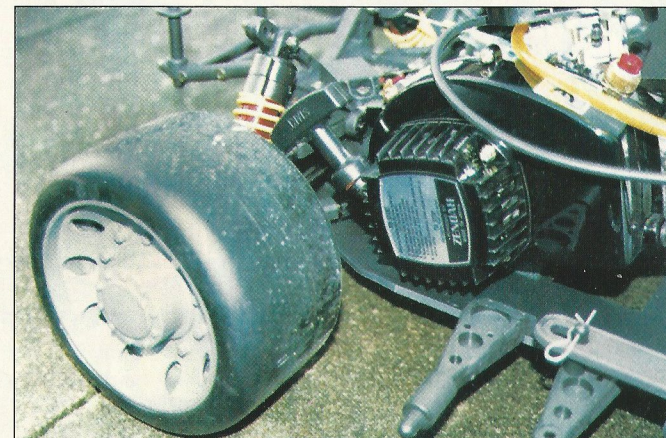
The truck has the first of a new generation of dual compound tyres.
