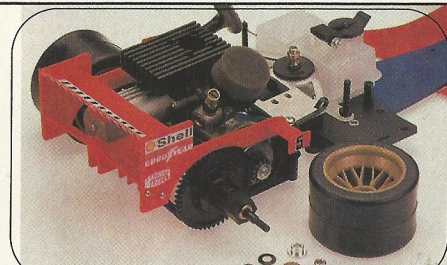
The pod rear end includes a ball differential
