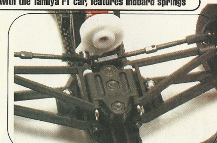
Front suspension is interchangeable with the Tamiya F1 car, features inboard springs
