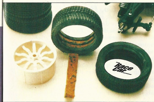
Left: The tyres are glued to the rims after the foam rubber inserts have been pressed into place.
