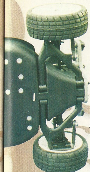
The Streetwise has in-board toe-in for better grip on rough tracks
