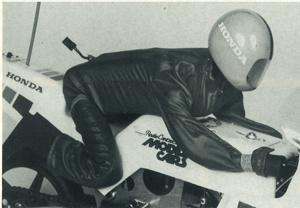
Above left: with bodywork and driver in place the 'Commando' cuts a realistic and exciting attitude: despite the Leakey quality of paint finish. Left: foam driver figure is encased in a single piece riding suit topped with a vac-formed helmet. The R/C battery pack is carried within the main body with the receiver connection exiting from behind.
