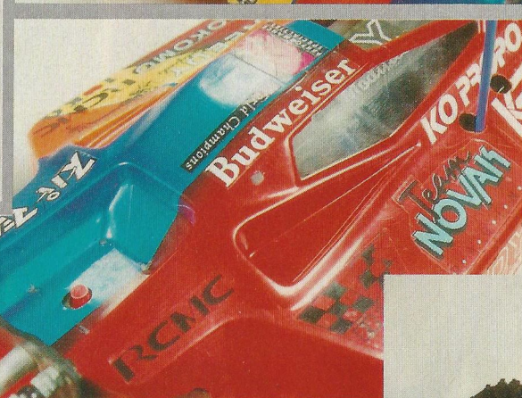
Craig uses the RCPS Turbo Mirage body on his RC10 - the body is very popular in the US. Note clever body post mounted through the body on the servo post.
