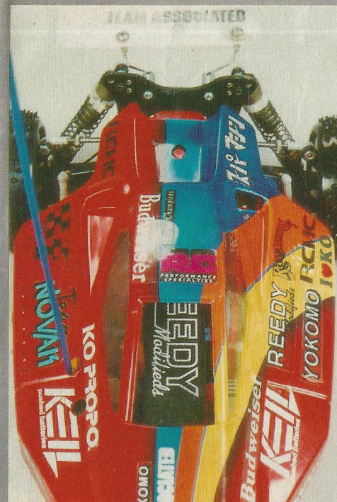
Standard Yokomo body and Associated wing fitted the 4WD. Note front window on the shell is cut out - mainly for the hot weather.
