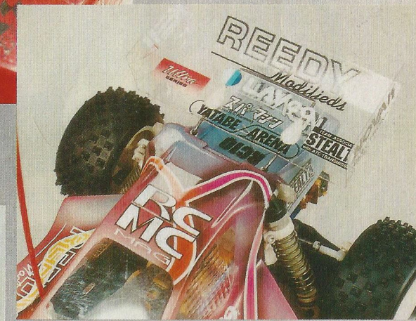
Craig uses the RCPS Turbo Mirage body on his RC10 - the body is very popular in the US. Note clever body post mounted through the body on the servo post.
