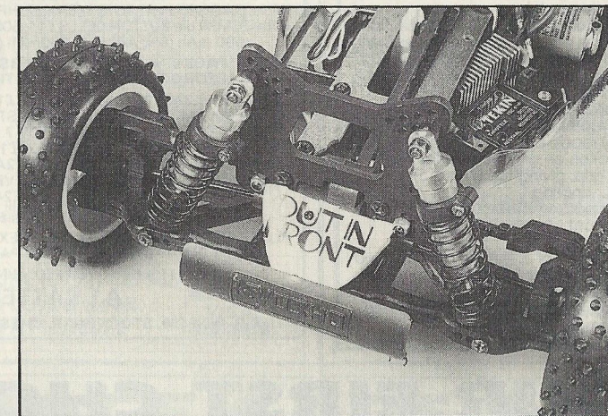
Super new front shock bracket is very light, neat and well made.
