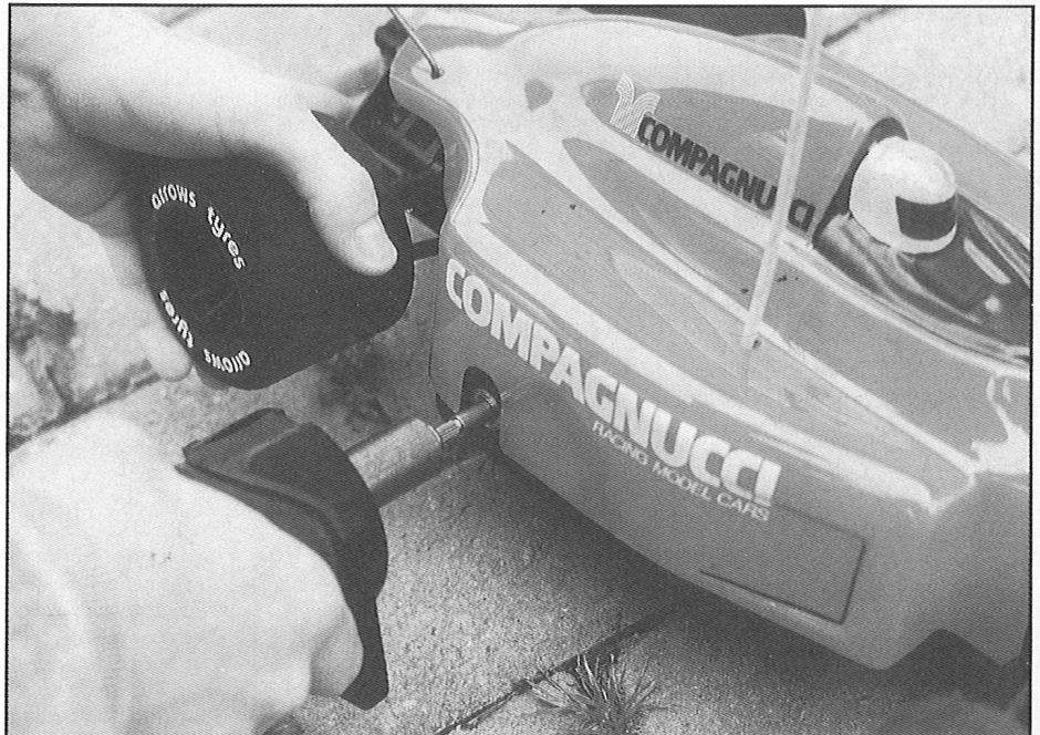
Above; Starting the car uses a clever system of a driver in the end of a standard starter motor. Left; Neat chassis consists of the plastic tub and neat moulded front bumper.
