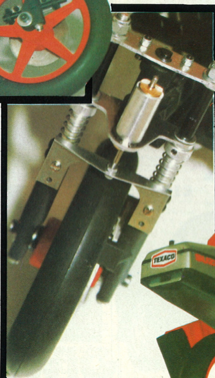
Above: Superbly engineered front forks employ dual springs and single damper.
