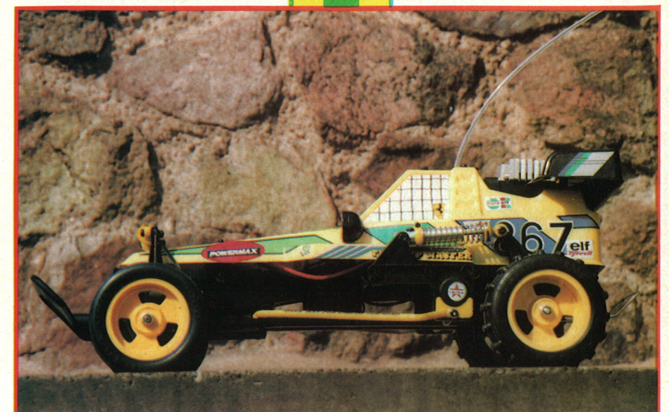
The Kangaroo is built around a girder chassis, everything else just bolts on.
