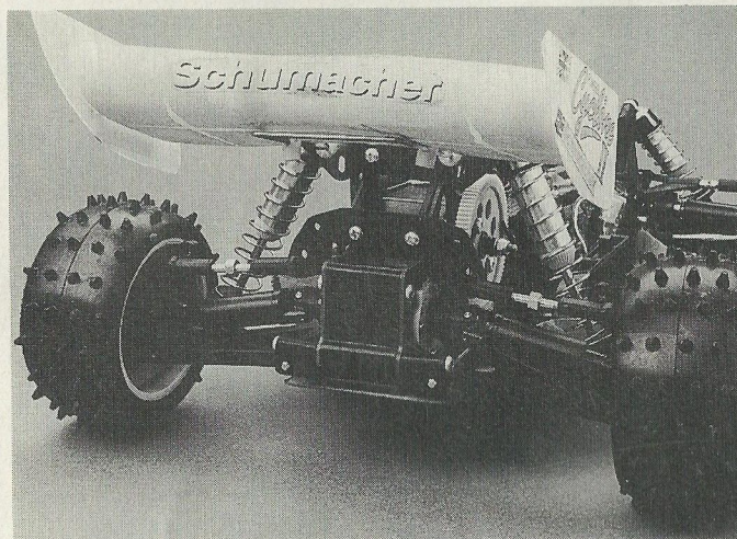
Wing mounts have changed from the early flimsy mount. Car is now wider at the rear.
