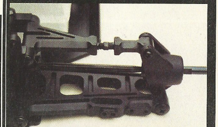
Adjustable camber using turnbuckles.
