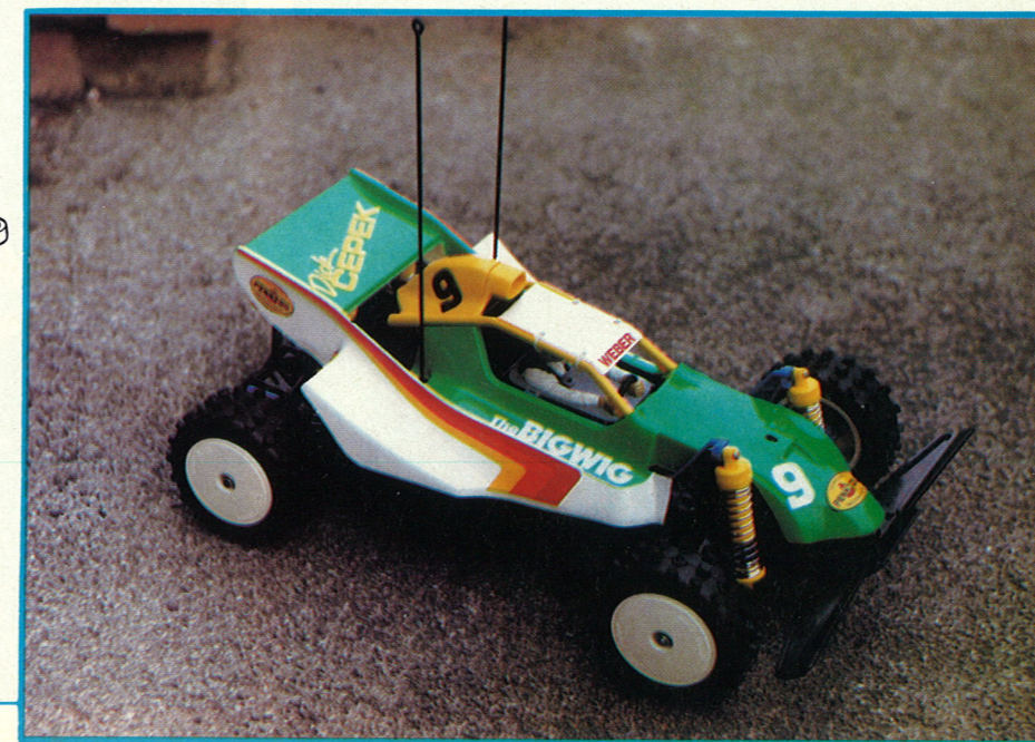
Rack and pinion steering virtually eliminates bump steer.
