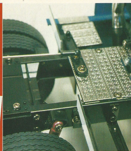
Above: Rear of cab. The aluminium panels were dry brushed with matt black to dull the chrome finish a little
