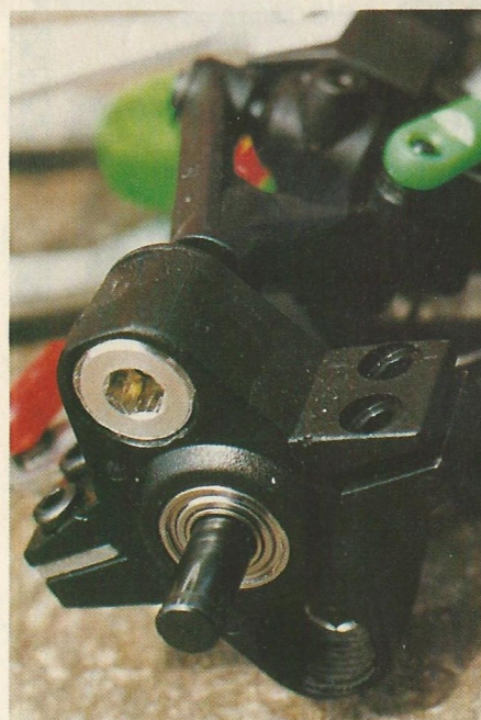
A front upright, showing the 'live' axle. The camber angle is adjusted by an allen key through the aluminium sockets.
