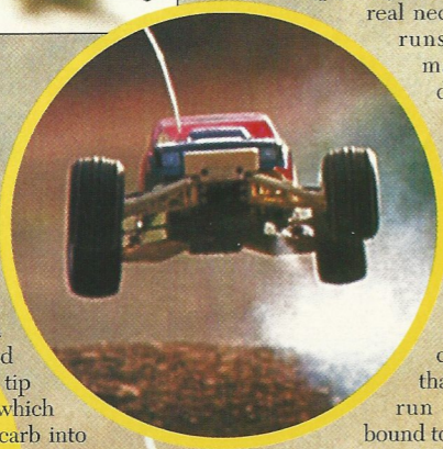
The front end follows conventional practice; a stout nylon lower wishbone with an adjustable upper link.
