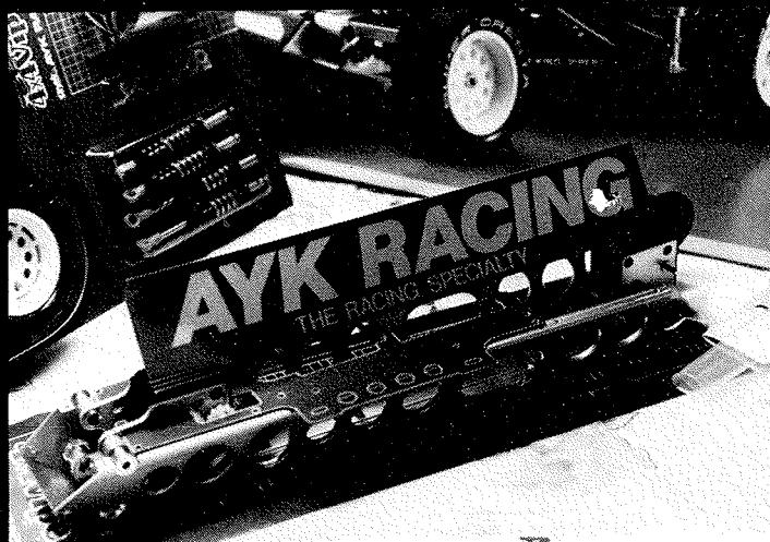
The unusual alloy monocoque frame chassis.
