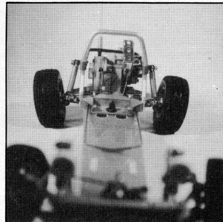
Steering and suspension units up front.
