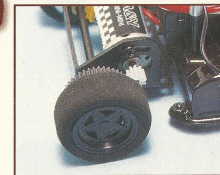
The rear mounted Mabuchi motor runs well with good duration but a hotter motor is available. Spur gear hides an efficient ball diff. Rear pod is flexible to give some rear suspension effect
