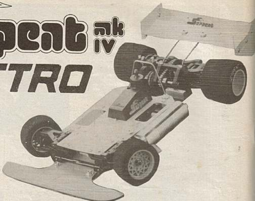
Right; impressive new Serpent "Quattro", a neat and tidy overall concept very nicely finished. Bottom left; ground level view of Quattro front end. Note the interesting hooked wire anti-roll bar system. Bottom right; underside view of rear wishbones, note spring around lower wishbone pivot pin. Front suspension upper wishbone shown below right. Below left; rear drive assembly complete - removable link can just be seen on the chain. Elite Models are to import the new Serpent.
