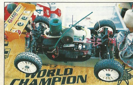
The Berganzoni Flash of Samuel Lenzi of Italy sported a Mugen tank, they don't break
