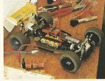
Rick Vehlow's Yokomo with centrally mounted ni-cads and glassfibre shock towers.
