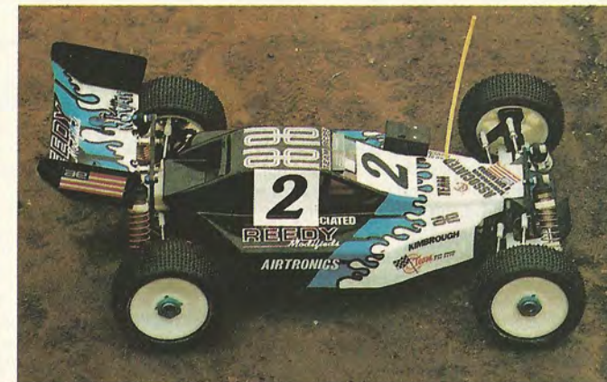
Brian Kinwald's maximum points scoring Yokomo. Note the SCR ni-cads, the extra PCB connected the Novak controller, the ballast to bring it up to weight and the controller heatsink through the windshield.
