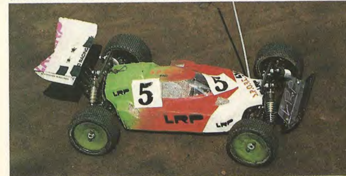
Thomas Jeschek's interesting 4WD car features torsion centre differential and unusual motor mounting position, all mounted in a home made carbon tub chassis.
