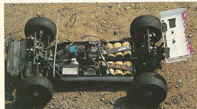
Thomas Jeschek's interesting 4WD car features torsion centre differential and unusual motor mounting position, all mounted in a home made carbon tub chassis.
