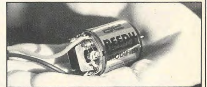
New wet ceramic Reedy modified, according to Mike this type of motor is a real step forward. It also performed extremely well at this meeting.
