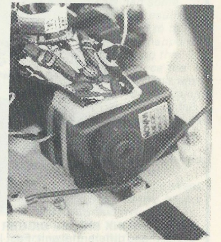
The Novak servo and radio receiver was used by almost every American driver. The centre Kydex spine was bolted and glued. This driver would have won concours if there had been one.
