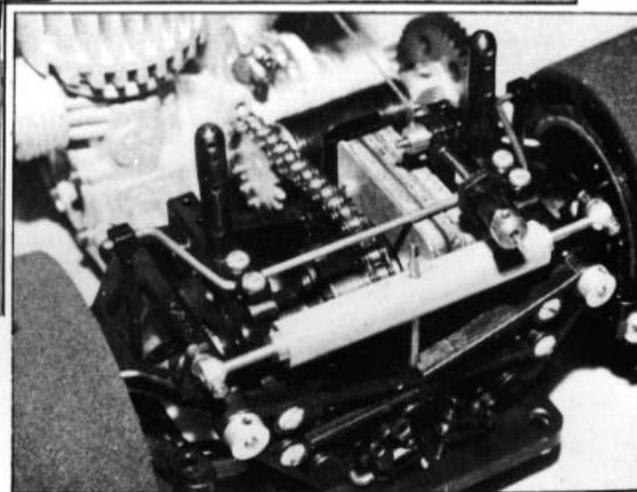
Above: the *Nova* rear-end is basically in standard *Alpha* Configuration with the exception of a single, dual purpose, damper across the rear. The damper can be converted from mono-shock operation to independent shock simply by removing the centre pin. Below: the *Nova* power pod is 'stepped' into the tube and held very firmly by three bolts passing right through the chassis.
